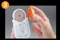
3. Apply new blade using blade change tool.
